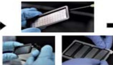
Lid affixed onto array case, filled with fluid, sealed, and loaded onto carrier.
