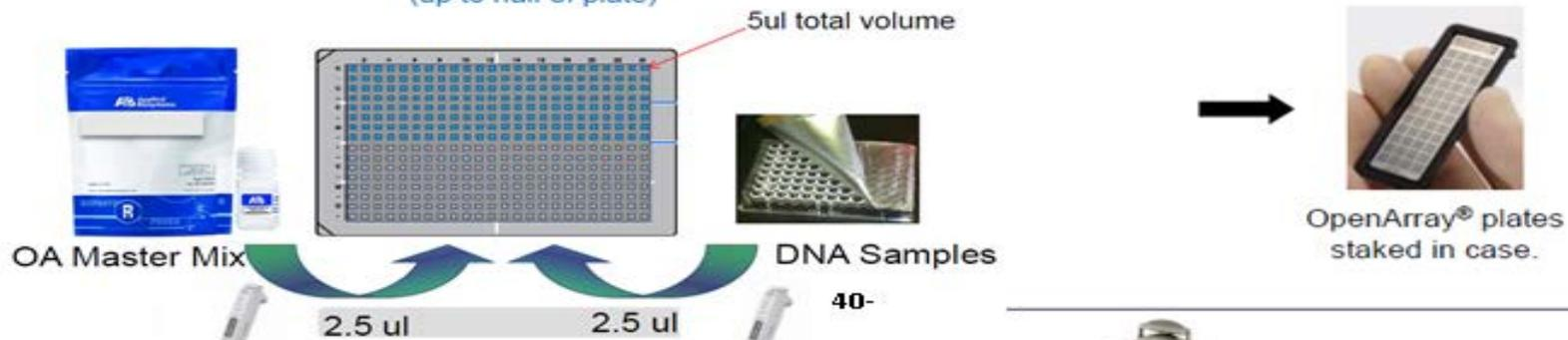
Samples and 2x Master Mix loaded onto the OpenArray® plate.
